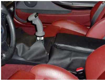
Figure 5. Central console with side stick from Stirling Dynamics Ltd.
