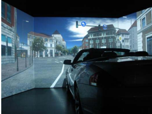
Figure 4. Static driving simulator
