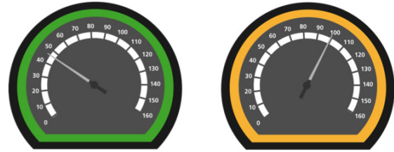
Figure 1: Example visualization of system3: EcoSpeedometer. Left (green) indicates an economical; right (orange) a wasteful driving behavior.
