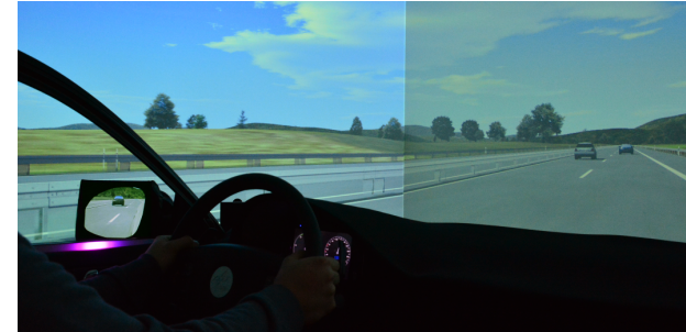
Figure 4: The final design for an overtaking scenario. If a car approaches on the left fast lane, a purple light moves towards the front left corner to display the distance. In addition its brightness adapts according to the assumed need for attention.
