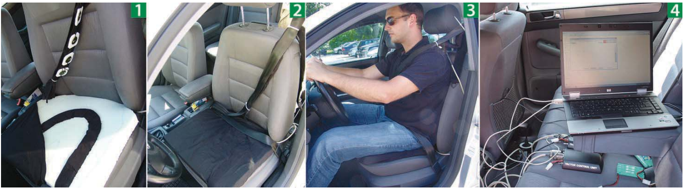
Figure 5: Hardware setting as used for the experimental studies. The vibro-tactile seat and safety belt interface with protective covers partly opened (1) and all closed (2), test person sitting in the car with both types of interfaces attached (3), tactile controller and data processing notebook in the back seat (4).
